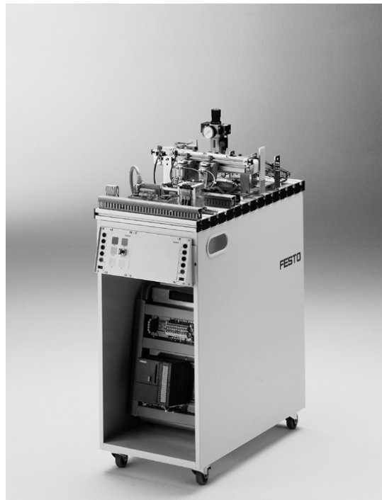
Sorting station with trolley, control console and PLC board
